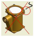
Strainers, according to models, come with raw body surface or with technical galvanic coating (nickel-plating). In case you wish, or have to, paint the strainer, please pay attention to leave the connection area unpainted, so that the earth connection cable can be in direct contact with bare metal, in order to avoid paint acting as insulation.
