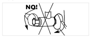
Carefully avoid to apply opposing torques to the valve/threaded end assembly. The anaerobic adhesive sealing the assembly may crack and void leaktightness. When threading the pipes into the valve, the retaining key should engage the clamping seat of the assembly on the same side of the threading pipe with respect to the stem and ball. The key clamping the valve should however always have a retaining function, the threading torque always being applied to the pipe.
